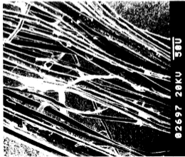
Fig. 13. Modern flax ( Linum usitatissimum ) fibres (50 micron scale)
